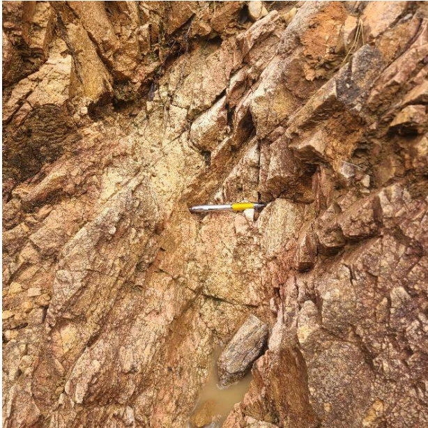
Figure 20 Quartzofeldspathic granite. Highly weathered feldspars disintegrating to clay
